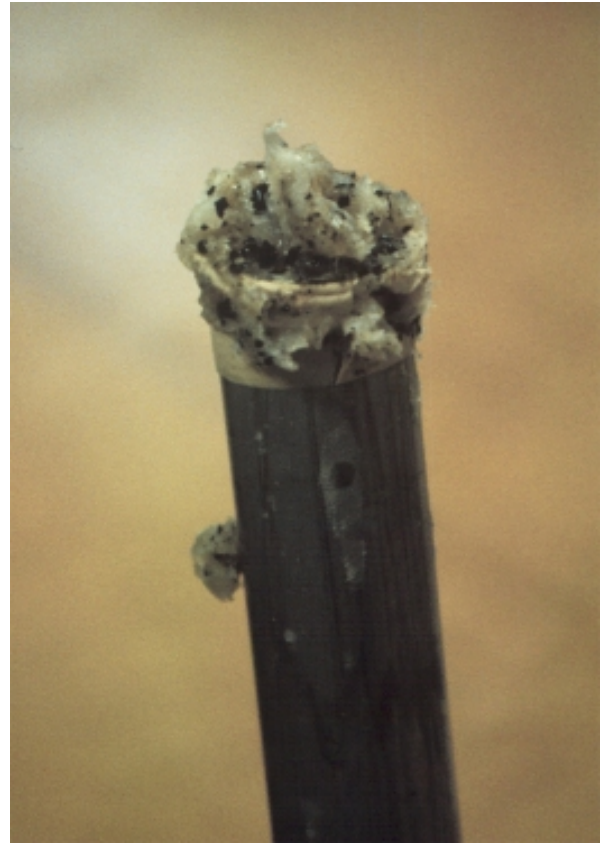
Figure 7. We utilized ABE’s controllability to take samples of volcanic glass using a wax-coring technique. We programmed ABE to stop at a selected spot, power down for a preset time, twist, then power up. The end of the core pole shattered glass on impact, and shards became trapped in the wax. A version that sequenced two poles (shown here) provided two samples per dive. The entire sampling sequence was captured on video still images
