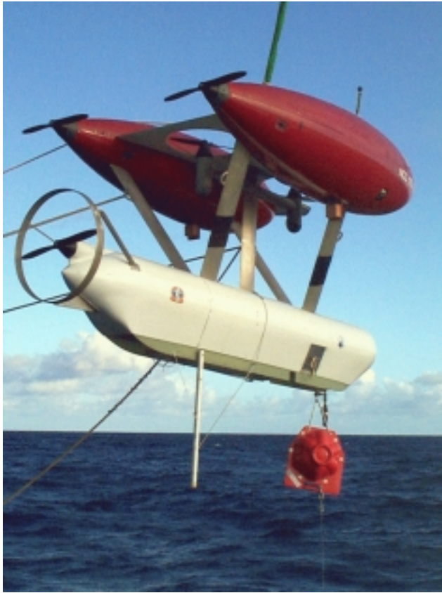
Figure 7. We utilized ABE’s controllability to take samples of volcanic glass using a wax-coring technique. We programmed ABE to stop at a selected spot, power down for a preset time, twist, then power up. The end of the core pole shattered glass on impact, and shards became trapped in the wax. A version that sequenced two poles (shown here) provided two samples per dive. The entire sampling sequence was captured on video still images
